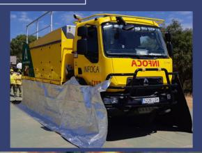
Patented system for the protection of fire fighters during critical situation of entrapment.
