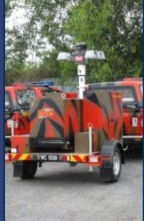
Pneumatic Telescopic mast with floodlight mounted to emergency response vehicle, to provide bright illumination during night time operations.
