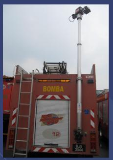
Mast can be installed at the external of vehicle, with suitable lower and upper fixing bracket.
