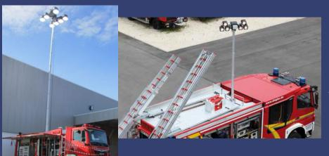
Mast can be installed at the internal of vehicle, with suitable roof fixing bracket.
