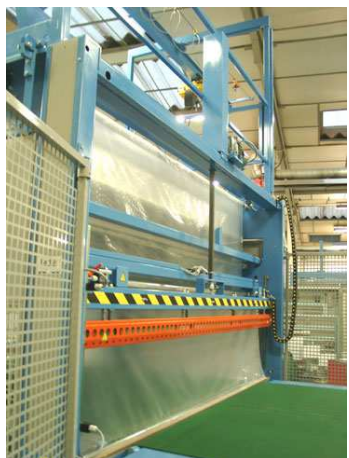
Wrapping unit with sealing bar
