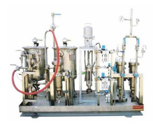
This system is consisting of some other systems which has the responsibility of Charging, Preparing, Filtering and Circulating of paint for paint lines.
