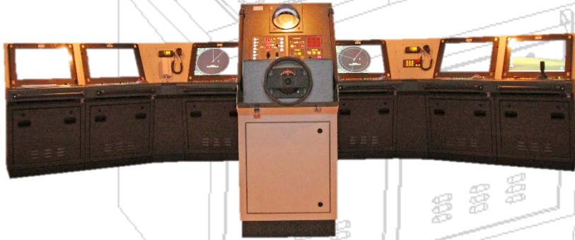
BRIDGE CONTROL CONSOLE
