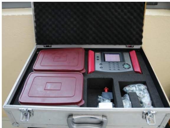
Portable data acquisition equipment, for field tests
