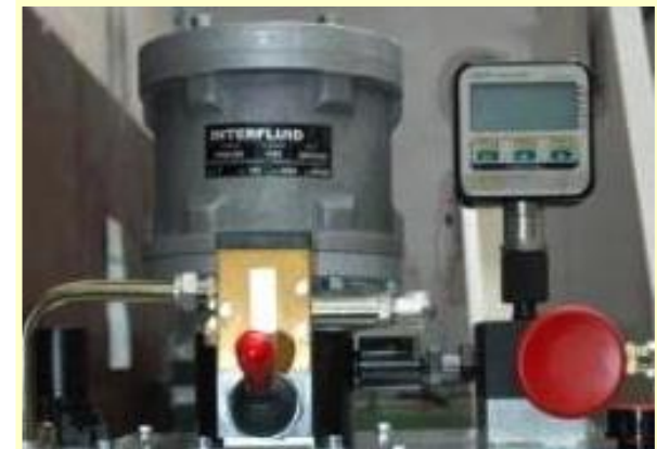
Burst test equipment 1850 bar
