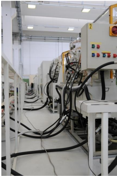
Centralized hydraulic circuit for all test benches
