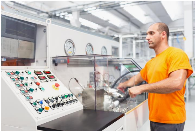
Improved functional test bench permanently connected to data acquisition software: 300 l/min / 550 bar
