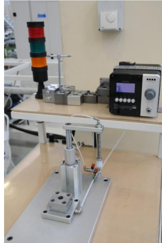
Leakage test with pneumatic equipment
