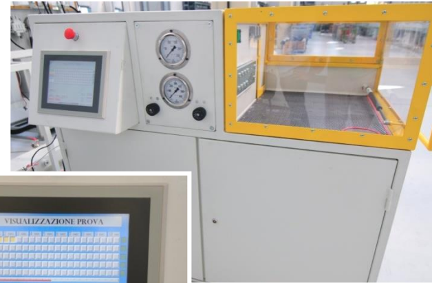
Endurance test equipment 700 bar
