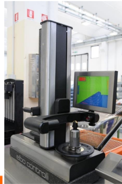
Machine to control sharpness and profile of the drilling tools and to fix them on the tool holder
