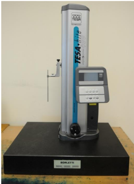
Machine to check cavities of the manifolds
