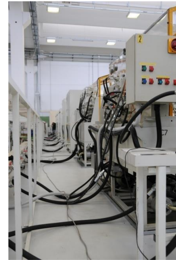
Centralized hydraulic circuit for all test benches
