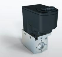
compared to other valve types that require constant electric power to hold its position. An integrated stepper motor enables precise adjustment of the ball design for accurate valve positioning and flow control. The optional absolute position sensor offers OBD (on-board diagnostic) functionality that eliminates the need for calibration on vehicle start-up and precise valve control through a LIN 2.x interface protocol.
