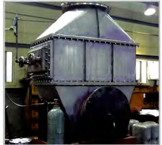
Heat Recovery Unit System
