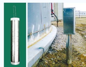
Wire-type ER sensor Installed beneath the AST
