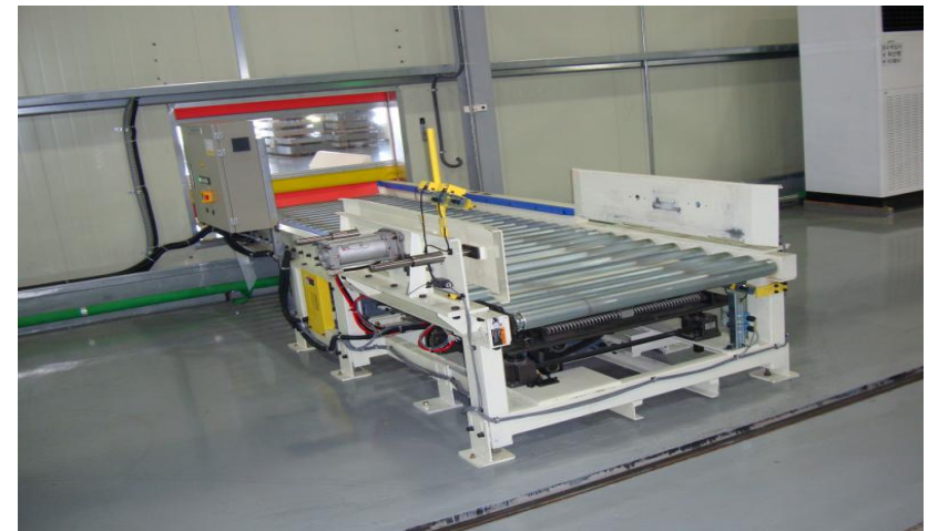
In-Out Let Conveyor System & Centering Device (3 ton)
