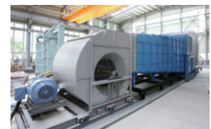
Test Facility (Open Type) of Air Cooled Heat Exchanger
