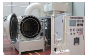
Test Facility (Closed Type) of Air Cooled Heat Exchanger
