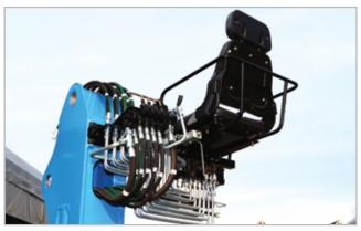
Two valves are setted for boom and outrigger operation seperatly. High capacity from two valves brings less pressure and low heat Boom valve with 6 sections & outrigger valve with 4 sections.
