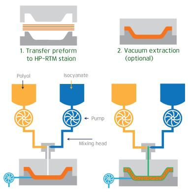
3. Resin injection/curing
