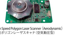
High Speed Polygon Laser Scanner (Aerodynamic)
