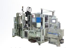
Crank Shaft Automatical Measuring Machines
