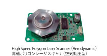
High Speed Polygon Laser Scanner (Aerodynamic)
