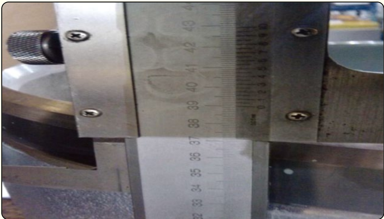
Photograph Explanation: Welding Type Butterfly Valve measurement inspection
