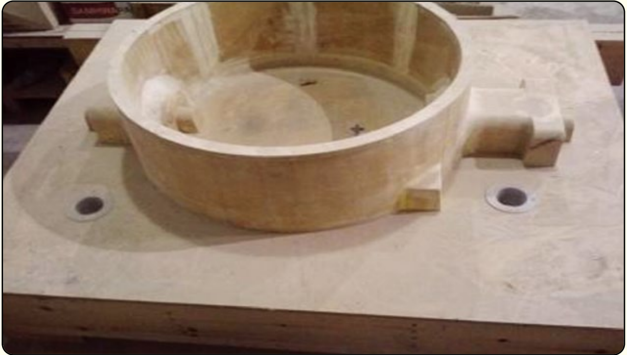
Wooden Model Photograph (specification 800A 1SET)
