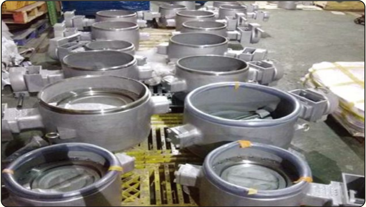
Photograph Explanation: Welding Type Butterfly Valve body processing
