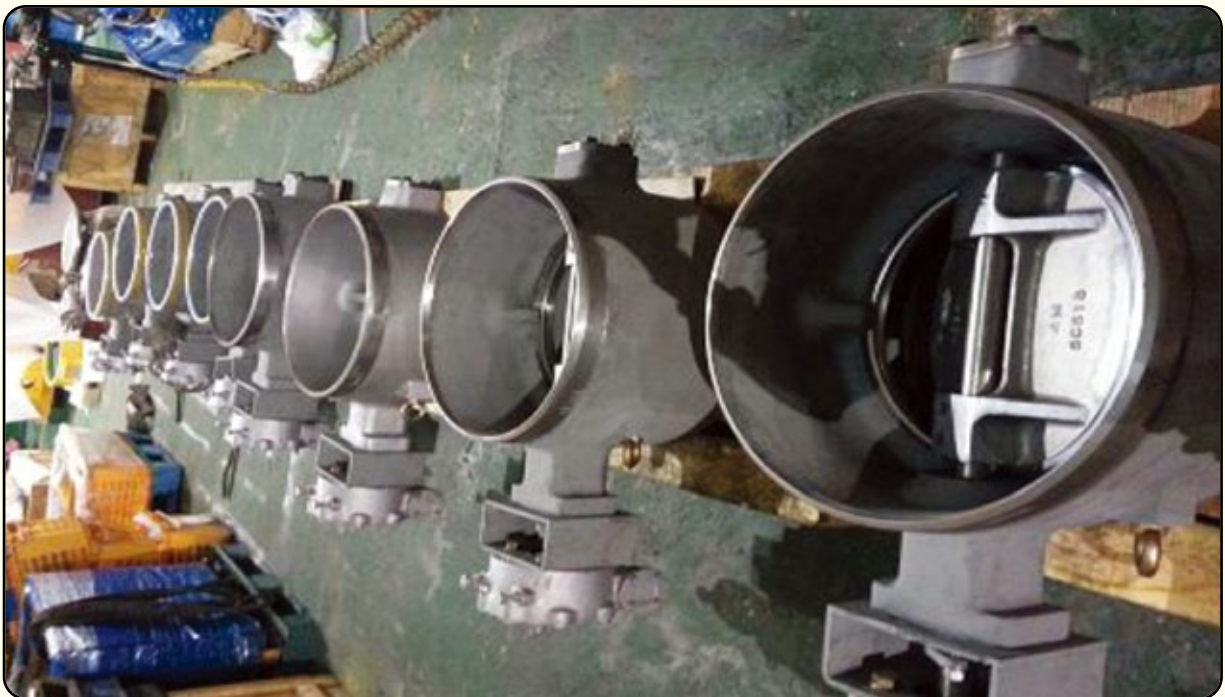
Photograph Explanation: Welding Type Butterfly Valve assembly
