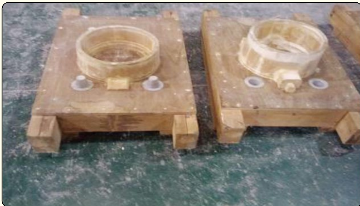
Wooden Model Photograph (specification 550A 1SET)
