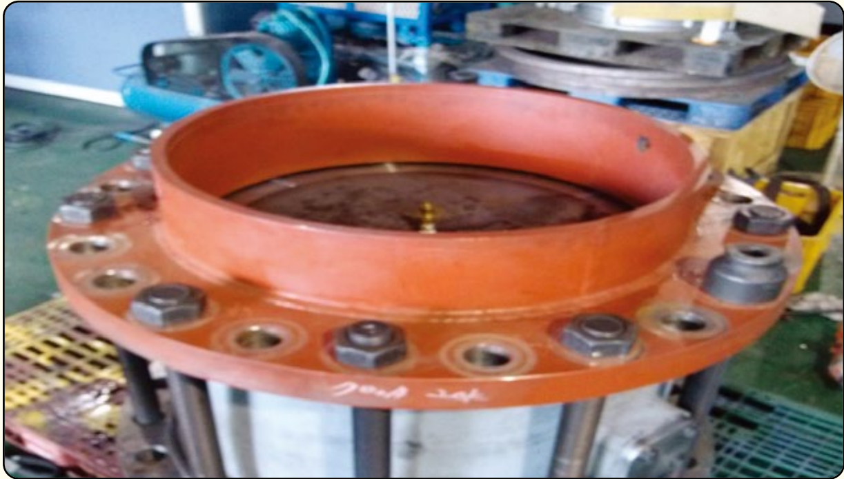
Photograph Explanation: Welding Type Butterfly body internal pressure test check
