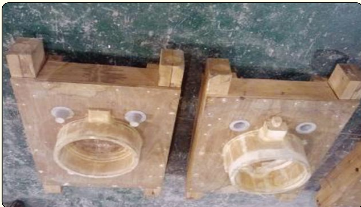
Wooden Model Photograph (specification 700A 1SET)
