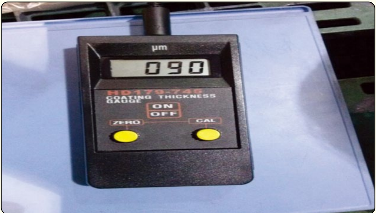
Photograph Explanation: Welding Type Butterfly Valve paint measurement
