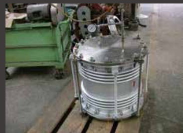
Hydro & burst test
