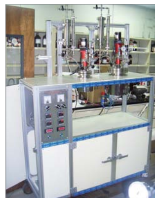
EO Gas Reactor System
