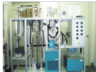
Supercritical Extraction System
