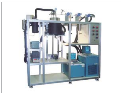
Supercritical Extraction System
