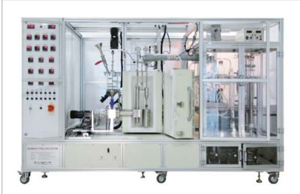
Continuous Fluidized Bed Reactor
