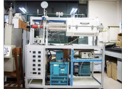
Supercritical Water Oxidation System
