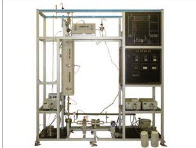
Continuous Supercritical Water System
