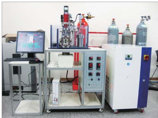
Hydrate Reactor System
