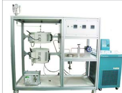
Supercritical Water System
