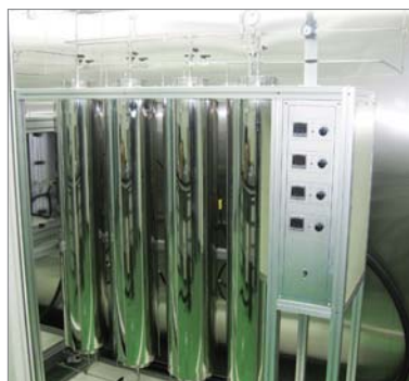
Gas Purification Column
