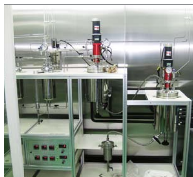
EO + PO Reactor System
