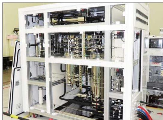
CO 2 Recovery System
