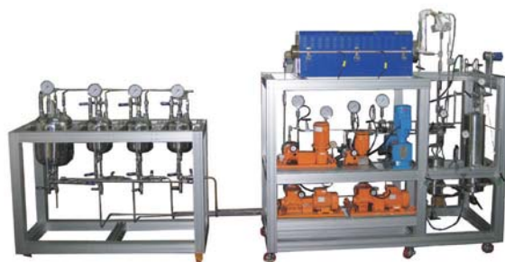
Continuous Supercritical Water System
