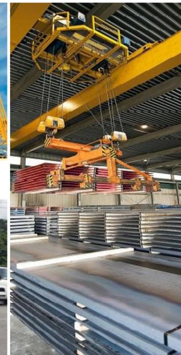
Overhead Crane with 2 hooked Hoist.
