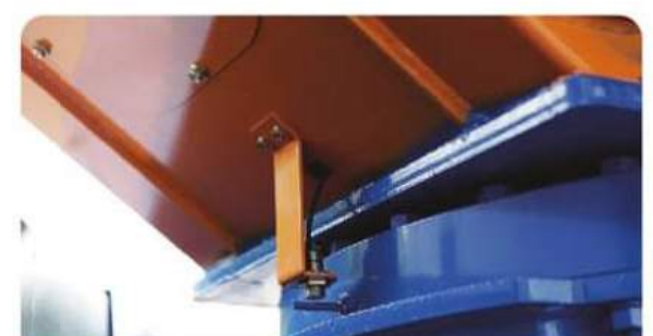
TURRET/BOOM ROTATION SENSOR
