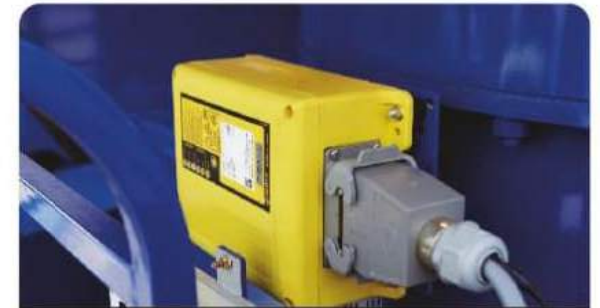
RECEIVER OF REMOTE CONTROLLER
