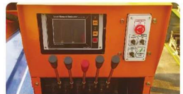
EMERGENCY STOP/ENGINE START / RPM / PTO SWITCHES
