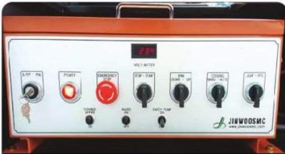
MAIN CONTROL PANEL BOX
