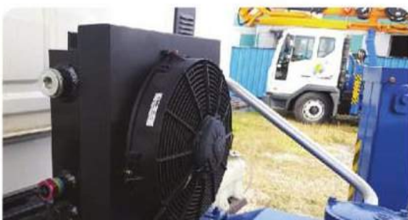
HYDRAULIC OIL COOLER
