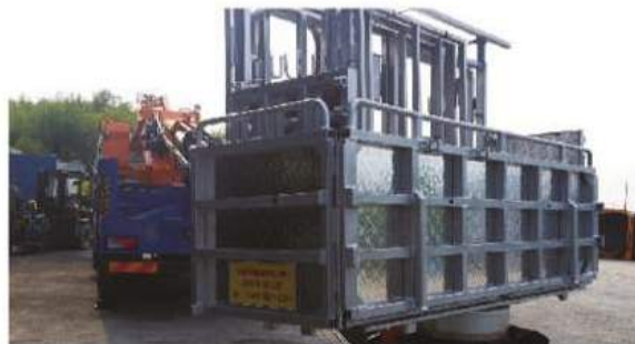
PLATFORM'S LOADING CAPACITY IS 400KG INCLUDING 3 PERSONS
