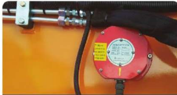
BOOM'S ANGLE SENSOR
