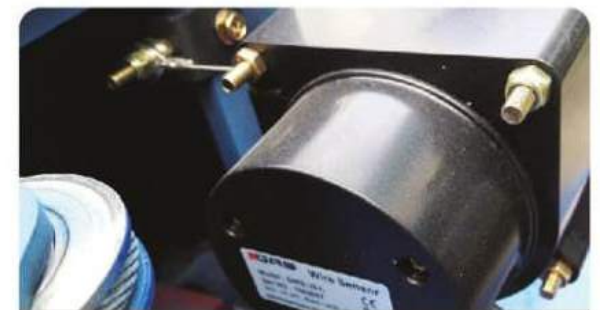
OUTRIGGER POSITION INDICATOR
