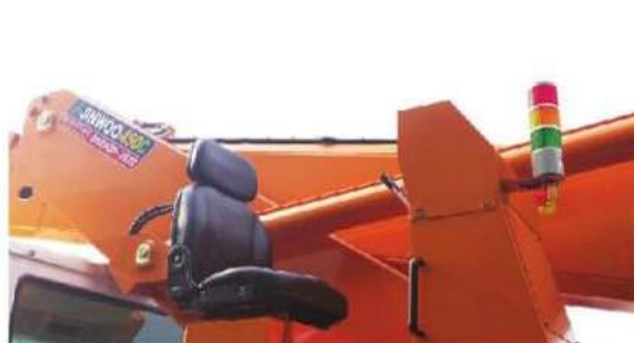
GROUND STATION CONTROL WITH OPERATOR SEAT
