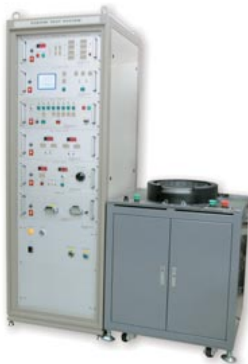
▲ Fig 9.1 shows an example of Stator Test Systems (Ass'y). It is automatically performing the required tests for the overall quality of products.
