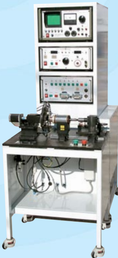
▲ Photo shows an example of Armature Test System. This System tests an armature of DC motor, and checks surge, hipot, 2 kinds of resistance between commutators, and Insulation. It can test 4,800 products a day (8 hours a day).
