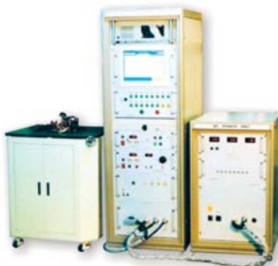
▲ Fig 8.1: DC MOTOR PERFORMANCE TEST SYSTEM ( KT- 217 ) Above Test Systems were supplied to various customers (SSE, car electric device manufacturers, etc).
