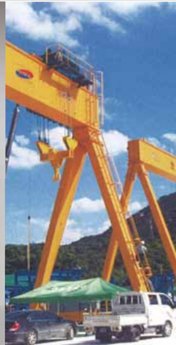
Mono Girder Gantry Crane (65ton) CCL KOREA in Uijeongbu (Span 28m*Height 14m) Max Capacity : 300 tons
