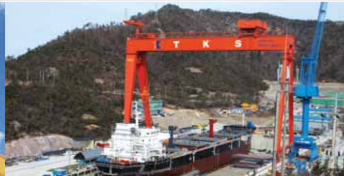
Goliath Crane for shipyard (600ton) TKS Shipyard in Yeonggwang (Span 100m*Height 80m) Max Capacity : 1500 tons
