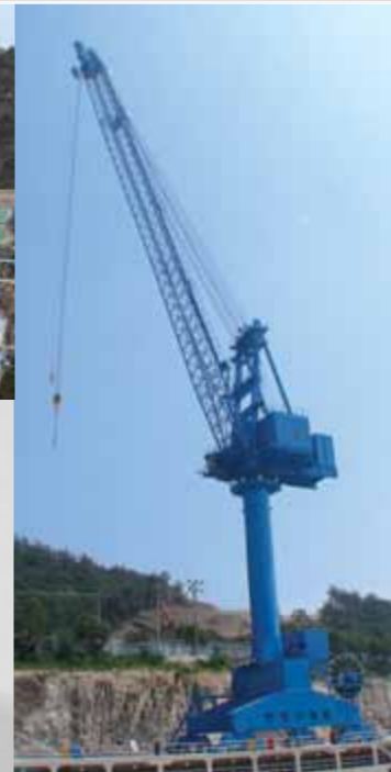
Level Luffing Crane for shipyard (40/5ton) TKS Shipyard in Yeonggwang Max Capacity : 100 tons
