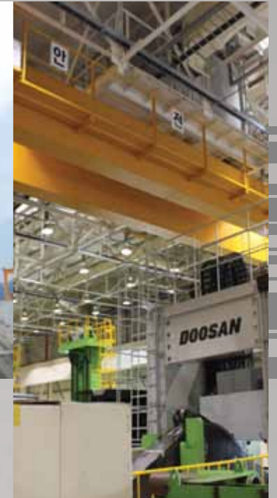
Double Girder Hoist Crane (100ton) Doosan Infracore in Gunsan (Span 24m*Height 12m) Max Capacity : 400 tons
