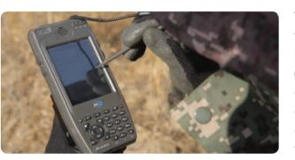
The Umpire PDA controls the soldiers during the training by Kill & Resurrect laser code. It can be used as the artillery and a cyber simulator (Chemical, Mine, and Obstacle zone). It could configure the MILES device before the training and download the training events stored in personal detector if necessary. It is used as a control tool for during the repair and maintenance as well.
