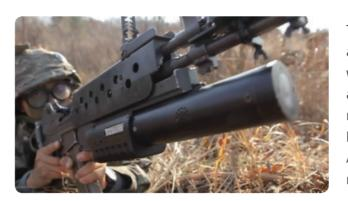
The Grenade launcher replicates the high-angle attack feature of actual weapon. Soldiers use weapon's leaf sight, quadrant sight, trigger, and normal elevation aiming as well. With high-resolution azimuth/elevation sensors in the launcher, the point of impact is calculated. Association with personal detector via WPAN makes the launcher disabled if the player is killed.
