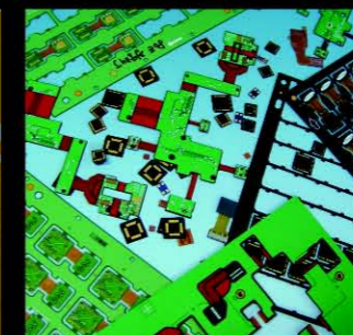
FPCB Body Cutting & Hole Drilling
