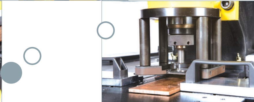
Busbar punching, bending, and cutting at the same time
