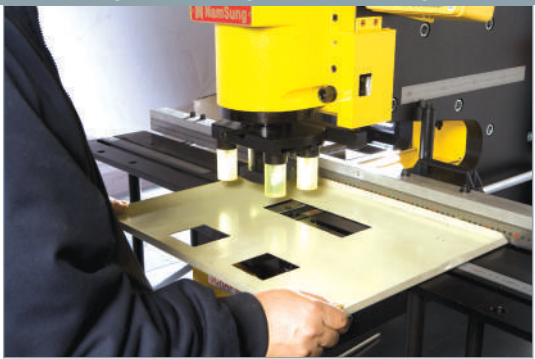
Busbar punching, bending, and cutting at the same time
