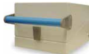
4921 RF Shield 700 to 1000 MHz / Typ. 90 dB 1700 to 2000 MHz / Typ. 90 dB 2000 to 2500 MHz / Typ. 85 dB 5000 to 6000 MHz / Typ. 80 dB
