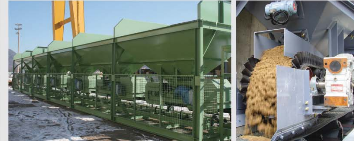
Creased belt conveyor for feeder units
