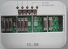
Plugging place for Plug-in type saw filter module
