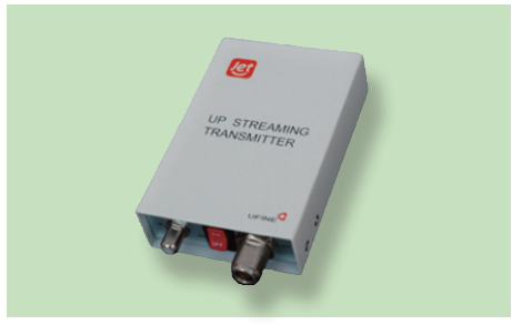
U/C (Up Converter) : Up Streaming Transmitter
