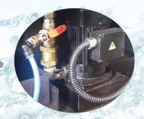
Assemble the cleaning line to the lubrication hose and open the cleaner's valve
