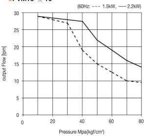
Total Efficiency  $\eta t = \frac{P \times Q}{612 \times Li} \times 100$  (%), Volumetric Efficiency  $\eta v = \frac{Qp}{Qo} \times 100$  (%)
