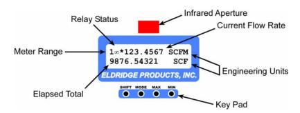
Meter Range — indicates the active meter calibration range (1–4), an exclamation point (!) indicates that the flowmeter is operating with menu item 212–Track Hold selected, a box ( $\Box$ ) indicates that the flow has exceeded the range of the 0–5VDC and 0–20mA output signals; Relay Status — indicates status of Relays 1 and 2 ( $\infty$  = de-energized, \* = energized); the Relay #2 symbol will be \* while operating in Multipoint mode.
