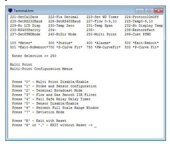
The 250 submenu includes a list of seven (7) control functions for use in programming the number of probes in your multipoint system, the number of sensors per probe, the sensor failure parameters, etc. All of these parameters are set up by the factory, but most may be adjusted as necessary to meet your specific requirements.
