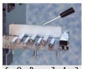
Straighten Unit」 Feeds wires without bending, range from AWG 12 to AWG 30.
