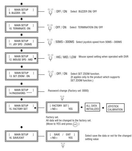
After factory set, the  $\mathsf{Tx}$  LED on the LCD screen flashing is not a malfunction.
