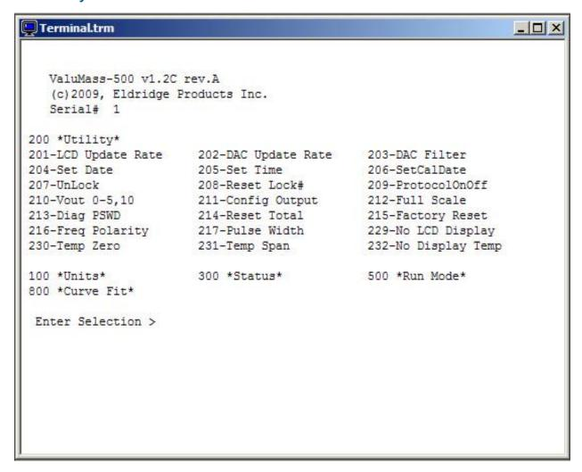
The 200 \*Utility\* Menu of the ValuMass<sup>TM</sup> flowmeter includes a series of submenu items which allow you to easily change a wide variety of microprocessor parameters, such as the display update rate, the internal date and time, etc. Values for timing functions are in millisecond (ms) increments.
