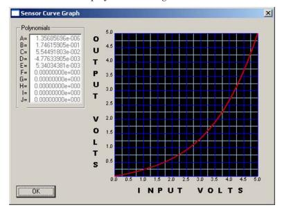
This screen shows the non-linear 0–5 VDC scaling of the bridge voltage and the Primary Coefficients used by the microprocessor to linearize the signal.
