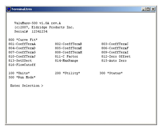
Although most settings are accessible by using the default user password of "9001", some of the parameters require a special password available only by contacting the factory. This has been instituted to prevent the accidental change of critical settings. The curve coefficients and MaxRange values should never be changed without direct factory instructions.
