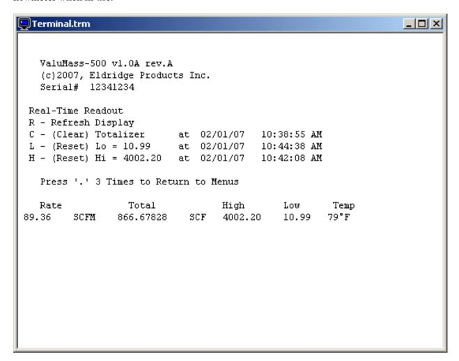
The Real-Time Readout commands are available while the flowmeter is in the basic Run Mode:
