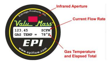
Infrared Aperture — allows infrared communications with EPI's LightWIRE™ I & II modules; Line 1 — Current Flow Rate is the real-time flow rate in currently selected engineering units; Line 2 alternates between —
