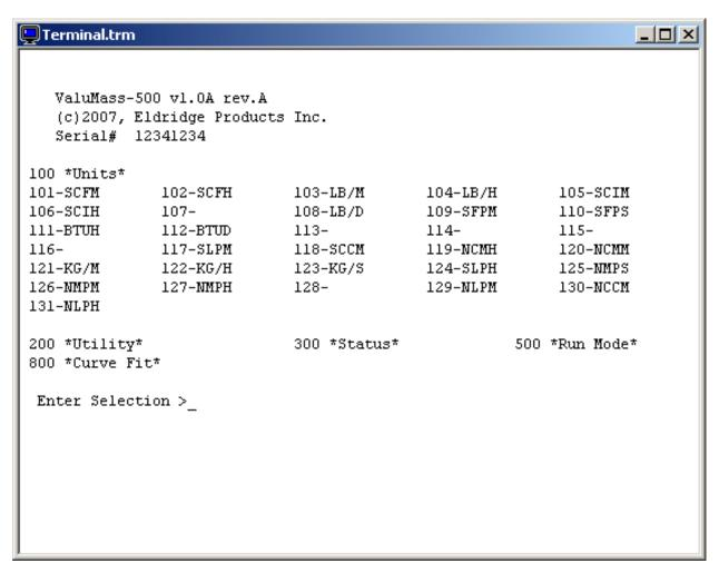
With the meter settings unlocked, type the menu number of desired engineering unit at the prompt and then press ENTER. The flowmeter will restart using new operational engineering units. The Full Scale and Maximum Range values are recalculated as part of this process (see menu items 212–FScale and 814–MaxRange).
