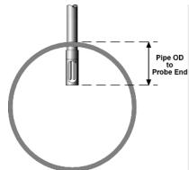
corrects the blockage effect created by inserting the probe assembly into the pipe to the depth listed.
