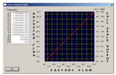
This screen shows the linear outputs and the corresponding flow rates. Adjustments made to the Full Scale, C-Factor, Zero Offset and Flow Cutoff will be reflected in this display.
