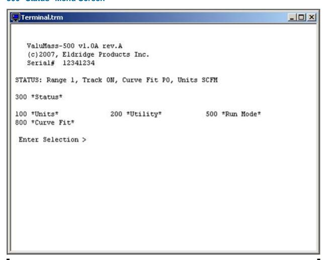
The 300 \*Status\* Menu is intended for use with the LCD display and does not present information on the PC screen.
