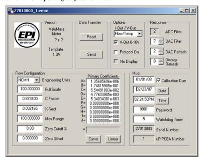
The various settings can be adjusted by either entering the new values directly into the data fields, by selecting from a dropdown list or by using the Up/Down arrows, depending on which values you are modifying. The values in grey fields cannot be modified by the user and are presented for reference only. When you have made any required adjustments, click the "Send" button to download the settings to the flowmeter.
