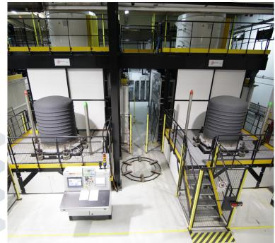
These furnaces are particularly adapted to Vapor Phase Aluminizing processes (VPA) of turbines blades but they can also be used as well for Vapor Phase Chromizing processes (VPC) as for pickling processes under HF gas (Hydrogen Fluoride), in the case of corrosion repairs and treatments (FIC Process – Fluoride Ion Cleaning).
