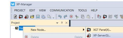
(3) Add XGT Pane node connected to PLC to be monitored on XP-Manger.
