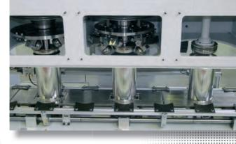
■ Top part produced on 3 stations for a fine adjustment.
