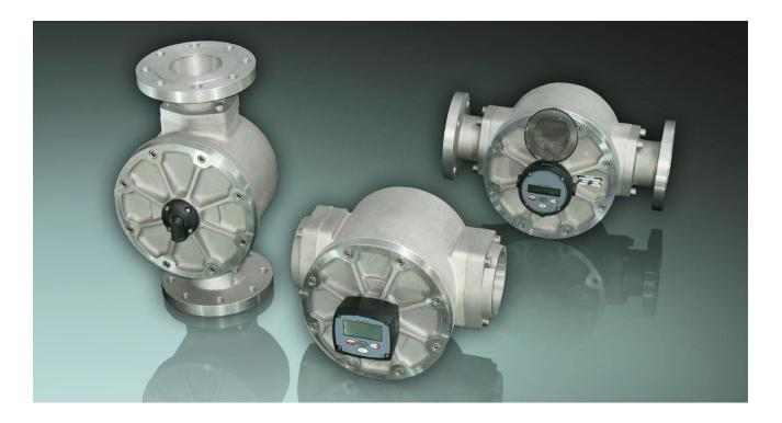
Fluidex series LOGF is a Positive Displacement Flow Meter with large capacity. The meters have two rotating gears in oval-shape. A fixed amount of the liquid passes between the gear teeth and through the meter after each revolution. The flow rate is identified by the number of shaft rotations. MLOGF are used in a wide range of applications where accurate measurement of liquid is required.
