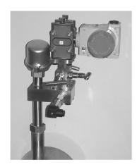
If desired, the deltaflow can be equipped with optional integrated pressure and temperature sensors.
