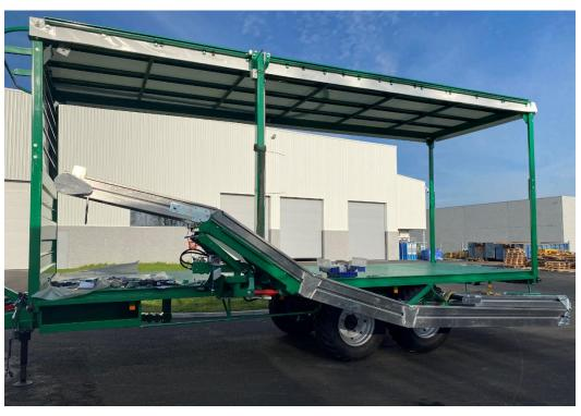
Swingable side belt for palox with a sliding mast for hydraulic movement
