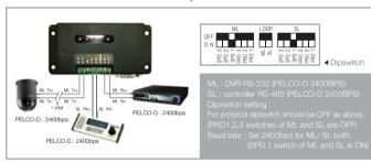
2. In case the protocol and baud rate is different between controller part (DVR and Keyboard) and PTZ camera
