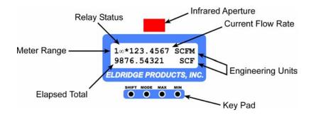
**Meter Range** — indicates the active meter calibration range (1–4), an exclamation point (!) indicates that the flowmeter is operating with menu item 212–Track Hold selected, a box ( $\Box$ ) indicates that the flow has exceeded the range of the 0–5VDC and 0–20mA output signals; a "D" indicates that the flowmeter is running the E-Log<sup>TM</sup> mode;
