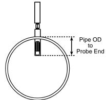
position or C-Factor may be required to improve the overall accuracy of the flowmeter readings. If an additional adjustment is necessary, the C-Factors below must be multiplied by the second correction to calculate the revised C-Factor. For example, if an adjustment of 0.975 must be made to the listed C-Factor for a  $\frac{1}{2}$ " probe in a 4" line (0.868), the revised C-Factor is 0.975 x 0.868 = 0.8463.
