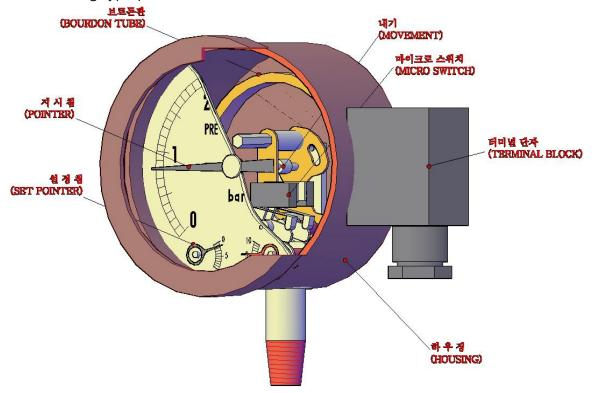
2) Indicating type pressure switch( 150mm )
