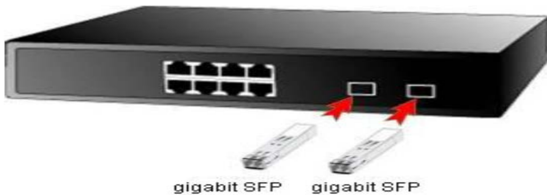
Plug-in the SFP transceiver
