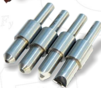
Replaceable inserts with natural diamond radius R2,R4,R6
