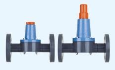
When the discharge pressure increases to more than a setting point due to choking the valve with debris or closing the valve, the safety valve will open automatically to relieve the pressure. Relief valve prevents pump and piping from damages.
