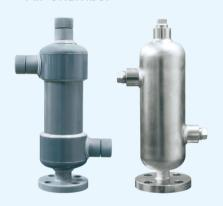
Reciprocating pump has a peculiar pulsation which results in vibration of piping and overfeed phenomena. Air chamber will be used to solve such problems caused by pulsation.
