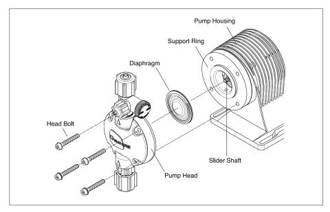
Assemble the pump head with head bolts, after positioning the Breath Hole of the Support Ring downward.
