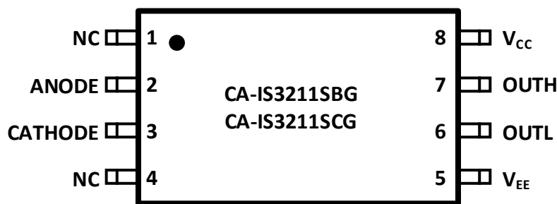
Figure 6-3. The CA-IS3211SBG/SCG Pin Configuration
