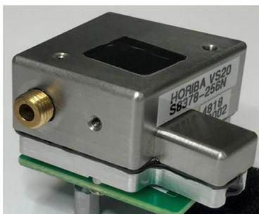
Spectrometer housing for S8378 sensor
