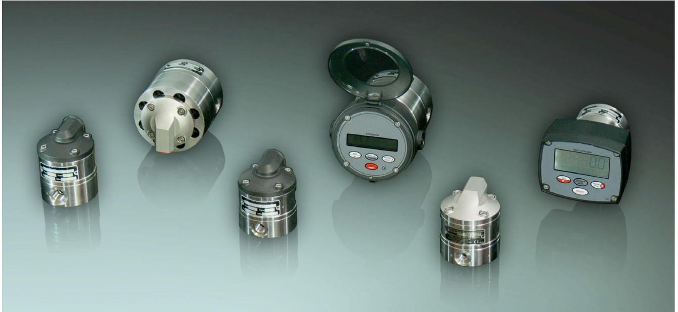
Fluidex series SOGF is a Positive Displacement Flow Meter with small capacity. The meters have two rotating gears in oval-shape. A fixed amount of the liquid passes between the gear teeth and through the meter after each revolution. The flow rate is identified by the number of shaft rotations during a certain period of time. The SOGF are used in a wide range of applications including the metering of fuel additives, corrosion inhibitors, emulsifiers and many others.
