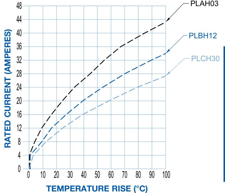
**TEST DETAIL:** Each curve was developed using individual connector bodies fully loaded with contacts. All power contacts energized through 12 awg wire. Temperature rise was measured in the contact mating area. Test was conducted with connectors in static air. Terminations of test connectors were straight compliant press-in to right angle (90°) solder. See page 4 for more information.
