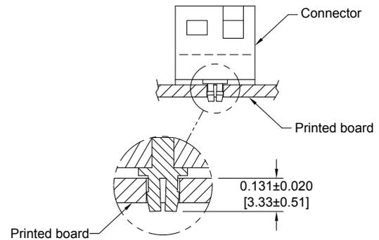
**MATERIAL:** Spring tempered copper alloy, tin plated.
