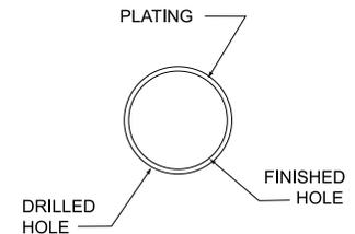
**COMPLIANT PRESS-IN TERMINATION CONTACT HOLE**
