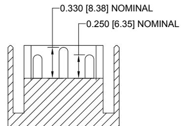
**MC610NS** and **MC612N** crimp contacts and **MC610NS** and **MC612N** solder cup contacts to be used for 0.330 [8.38] nominal mating length. **MC610NS-228.2** and **MC612N-228.2** crimp contacts and **MS610NS-228.2** and **MS612N-228.2** solder cup contacts to be used for 0.250 [6.35] nominal mating length.
