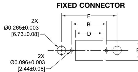
**NOTE:** Panel thickness may impact the orientation of mating end of blind mate pin. Shimming between the panel and the head of the blind mate pin may be necessary to minimize tilt of the blind mate system. Contact technical sales for additional technical information.
