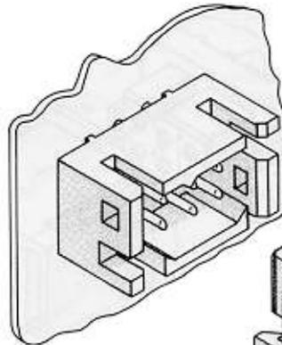
PLB06M300A1 Straight solder or PLB06M92ST20A1 Compliant termination press-in
