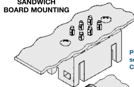
PLB06M300A1 Straight solder or PLB06M93ST30A1 Compliant termination press-in
